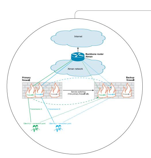
The Atman Firewall service is based on a pair of clustered Fortinet FortiGate appliances – a primary firewall, and a back-up firewall that takes over the traffic control when the first one is unavailable.
